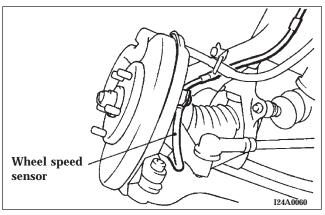
3. After driving on snow or icy roads, remove any snow and ice that may have adhered to the wheel areas. When doing this be careful not to damage the wheel speed sensors and cables located at each wheel on vehicles equipped with an anti-lock braking system.
